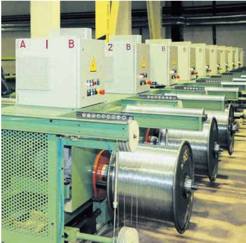
UNINSULATED WIRES for OHPL
